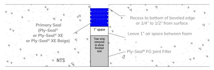
The Ply-Seal® Joint System with Ply-Seal® FG offers a convenient, durable, waterproof expansion joint system. The Ply-Seal® FG is a full depth, waterproof seal forming the joint gap as the contractor pours the concrete. The top section of the Ply-Seal® FG is removed after concrete cure at a prefab tear strip section, creating a cavity for the primary seal: Ply-Seal®.
