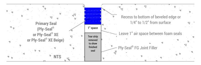
The **Ply-Seal**<sup>®</sup> **Joint System** with **Ply-Seal**<sup>®</sup> **FG** offers a convenient, durable, waterproof expansion joint system. The **Ply-Seal**<sup>®</sup> **FG** is a full depth, waterproof seal forming the joint gap as the contractor pours the concrete. The top section of the **Ply-Seal**<sup>®</sup> **FG** is removed after concrete cure at a prefab tear strip section, creating a cavity for the primary seal: **Ply-Seal**<sup>®</sup>.
