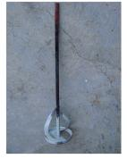
This "Paint" mixing paddle draws in excessive air into mixed A and B components. This unit is not recommended for urethanes.
