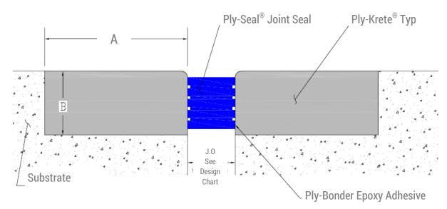
**Ply-Krete**<sup>®</sup> Joint Systems consists of **Ply-Seal**<sup>®</sup>, a waterproof joint seal, and **Ply-Krete**<sup>®</sup>, a durable, fast-setting, elastomeric concrete nosing material. This easy-to-install system requires minimal downtime, making it a convenient joint system for bridge joints.
