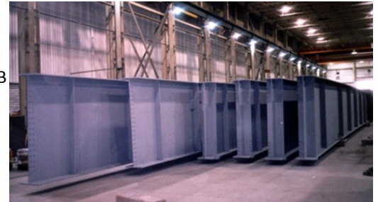
Bridge Girders coated with WB HRZS Single Coat System
