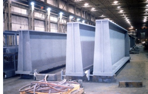
Bridge Girders coated with WB HRZS Single Coat System
