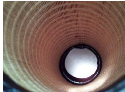
Rigid Foam Adhesive on Filter End-Cap
