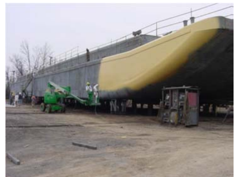
Inland Barge, WB HRZS ® Duplex Systems (Topcoats Include Polyaspartic, Polysiloxane, Mastic Epoxy Non-Skid)
