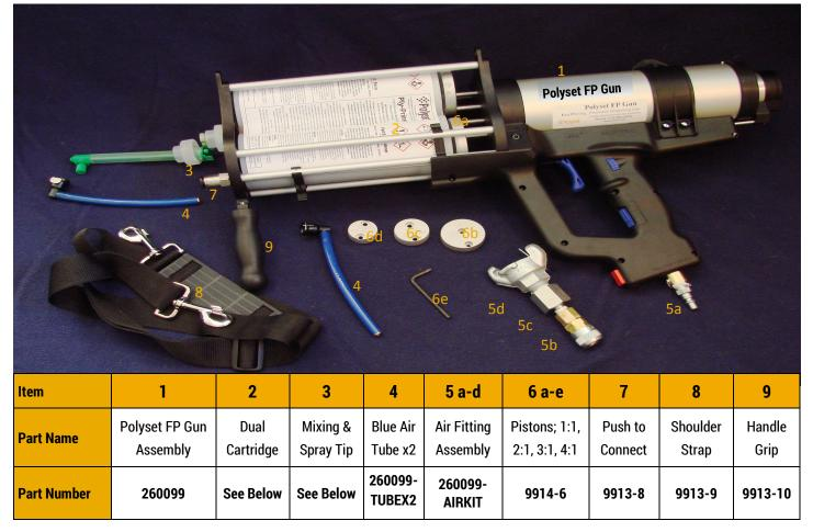
The **Polyset FP Gun** is designed to facilitate the installation of the **Ply-Krete® Joint Systems**. Designed as a pneumatic dispensing unit, it dispenses, mixes, and sprays our products from dual cartridges onto the prepared surfaces, eliminating the need to "paint" on the primer or bonder. This gun drastically saves labor and product cost while reducing installation time. Priming a joint may be reduced from 60 minutes to 6 minutes without mixers or brushes.
