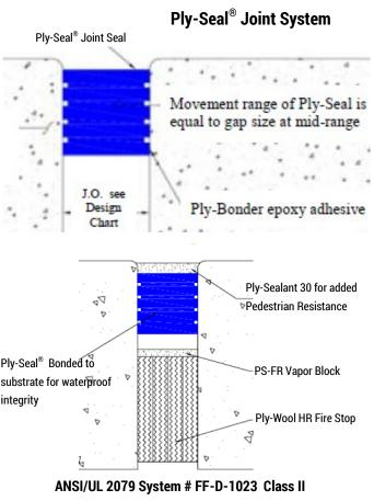
3-Hour Fire Stop with Added Waterproof Joint Seal
